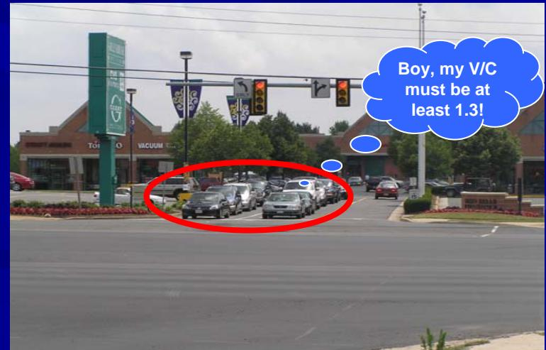
.....even the lower volume critical turning movements exiting from the high volume roadway can experience significant delay causing traffic congestion....
