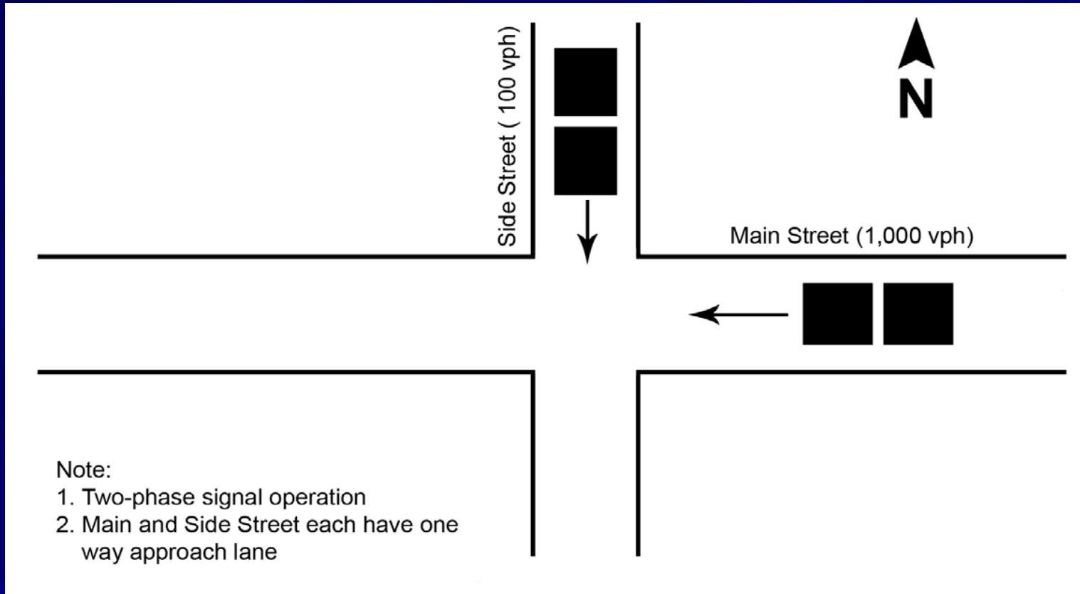
\* [Cycle Length = 100 seconds, two phase operation, 3 seconds clearance time per phase; main street 1,000 vehicles per hour, one lane, one-way; minor street 100 vehicles per hour, one lane, one-way.]
